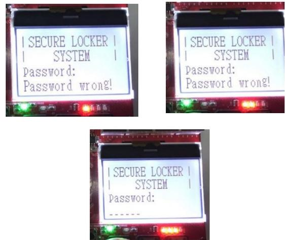
Fig. 7 LEDRs light in sequence while error detected
