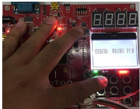
Fig. 8 Error message and buzzer for wrong pin activated
