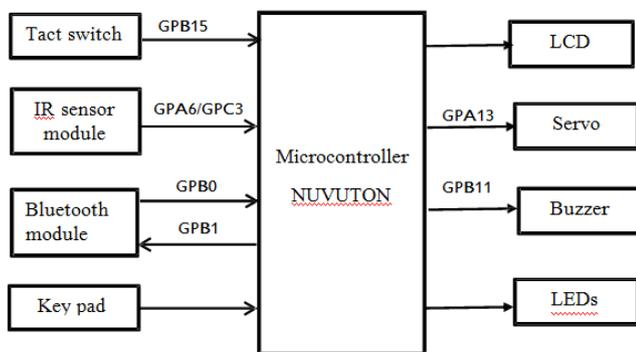
Fig. 1 Block diagram of the Secure Locker System
