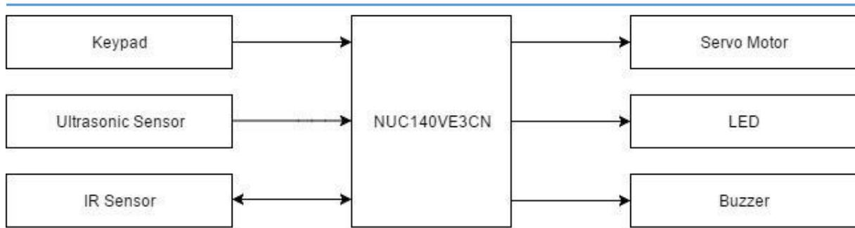
**Fig. 3.** Block diagram of Smart Locker System.
