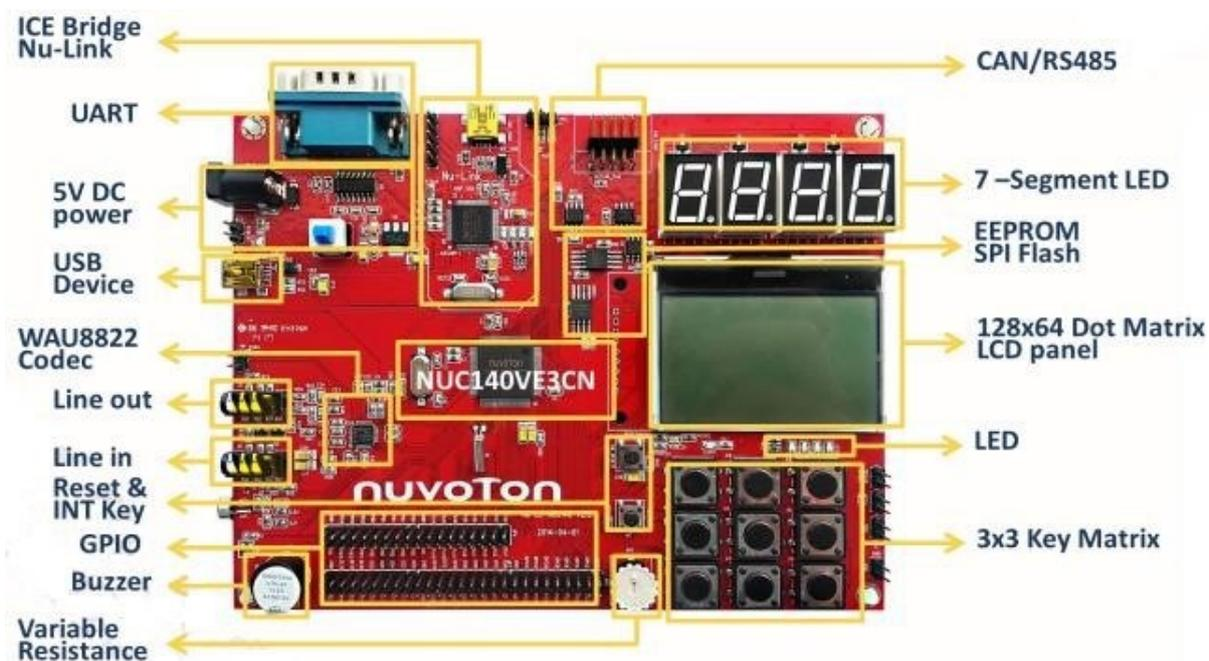
**Fig. 1.** Nuvoton NUC140VE3CN board with the function of block tagged
