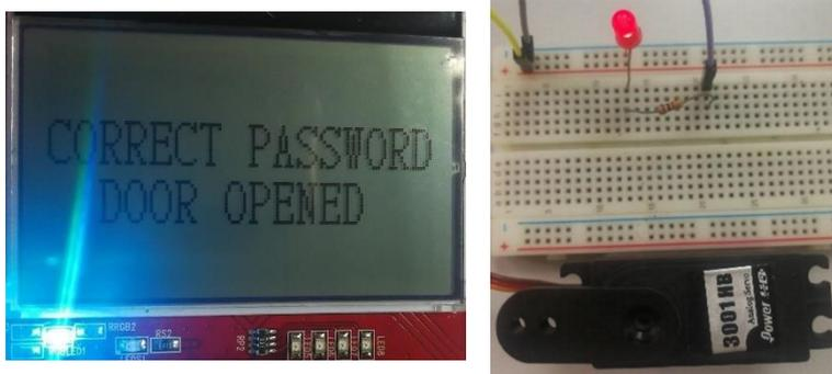
**Fig. 5.** Correct password enter and servo will opened the door
