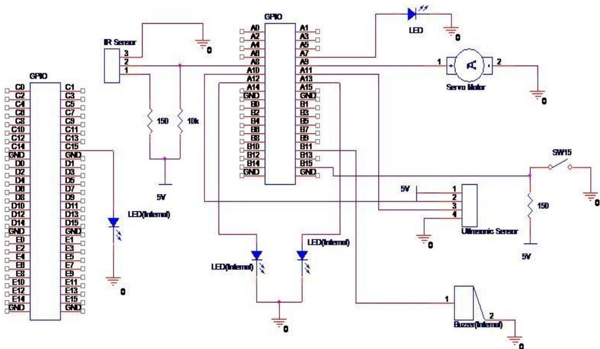
**Fig. 2.** Schematic circuit designs of Smart Locker System.
